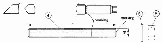
Marking: Works symbol / Length of threaded rod. or: Works symbol Property class 8.8 additional •.
